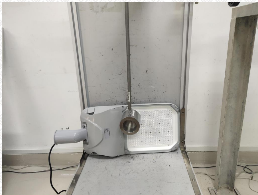
Photo 3: IK08 test of model AOK-150WiL02-NV-L3-00-40
