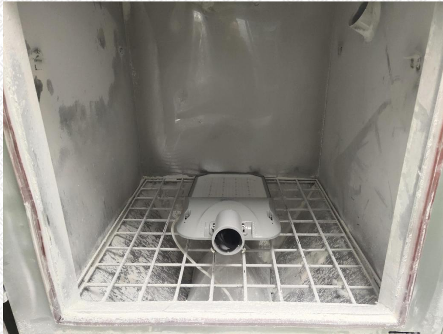
Photo 3: IP6X test of model AOK-150WiL02-NV-L3-00-40
