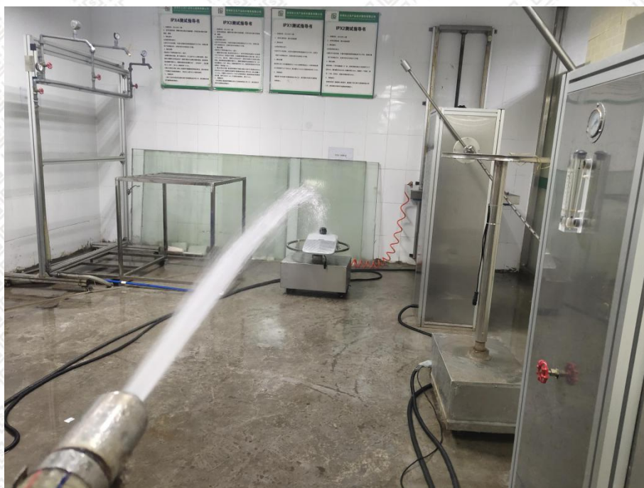
Photo 4: IPX6 test of model AOK-150WiL02-NV-L3-00-40
