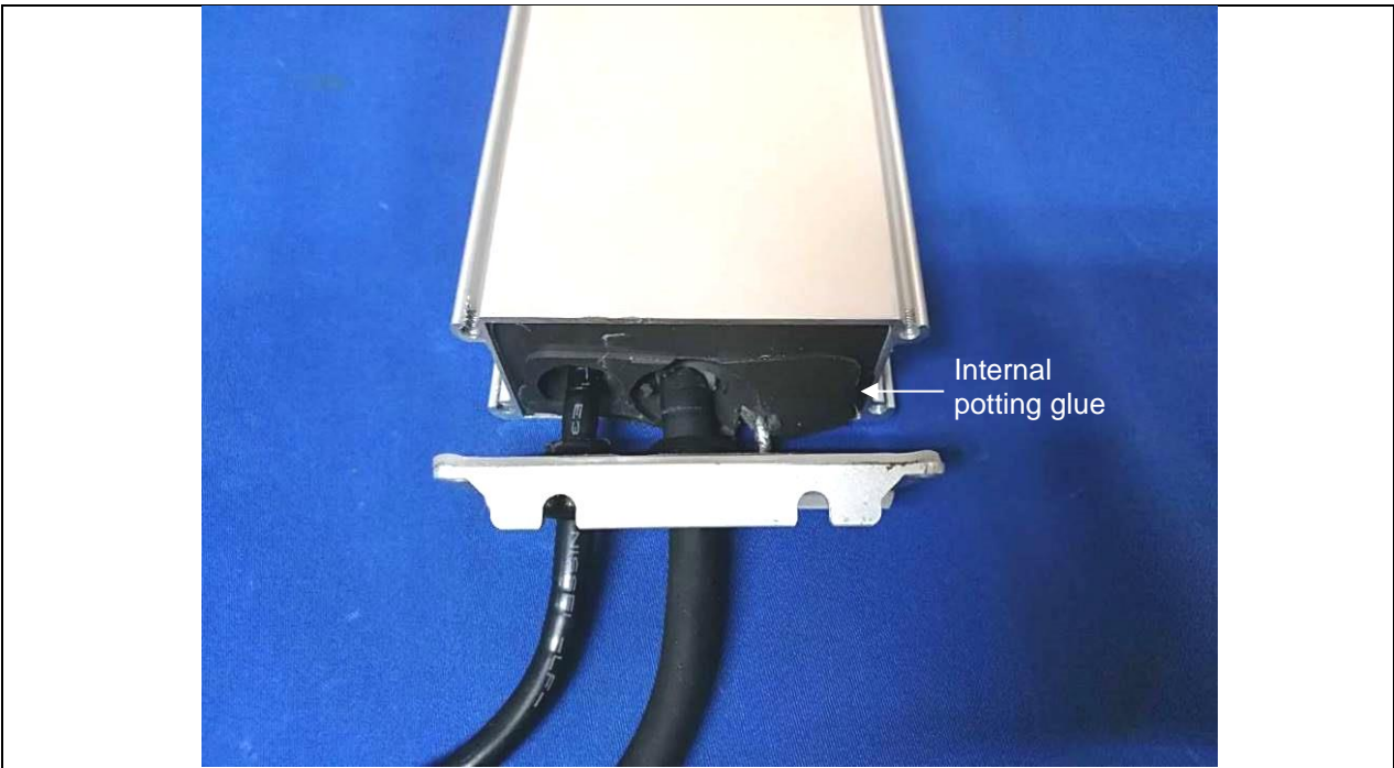
Details of: LED driver view SS-50VP-56DH
