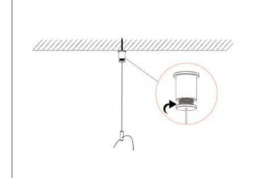
4. Screw the fixed female head at the bottom of the hanging rope into the installed male head of the lamp, as shown below:
