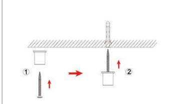
3. Screw the fixed male head at the top of the hanging rope into the fixed female head, as shown in the figure below:
