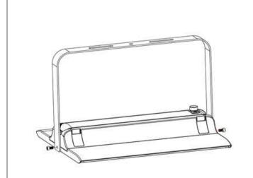
3. The bracket and fixture body are locked with screws as shown below:
