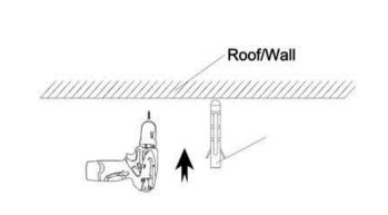
2. Drill holes with tools and insert the plastic expansion tube. Combine the self-locking screw with the fixed female head and screw in the plastic expansion tube at the same time, as shown below:
