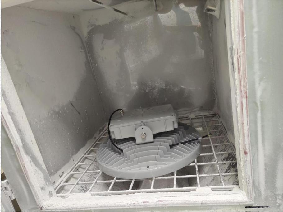
Photo 4: IPX6 test of model AOK-580WiNS-NV-L5-00-4080-BN-P
