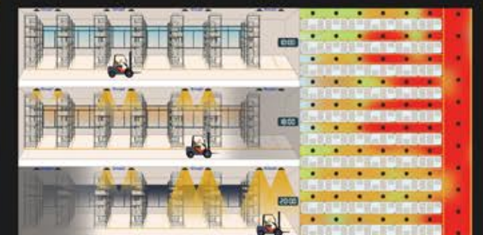
Motion (3-step dimming) + Daylight Sensor (constant illuminance)
