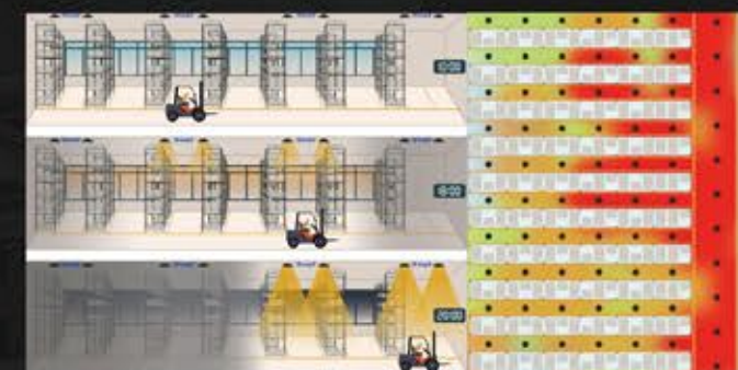
Motion (2-step dimming) + Daylight Sensor (constant illuminance)
