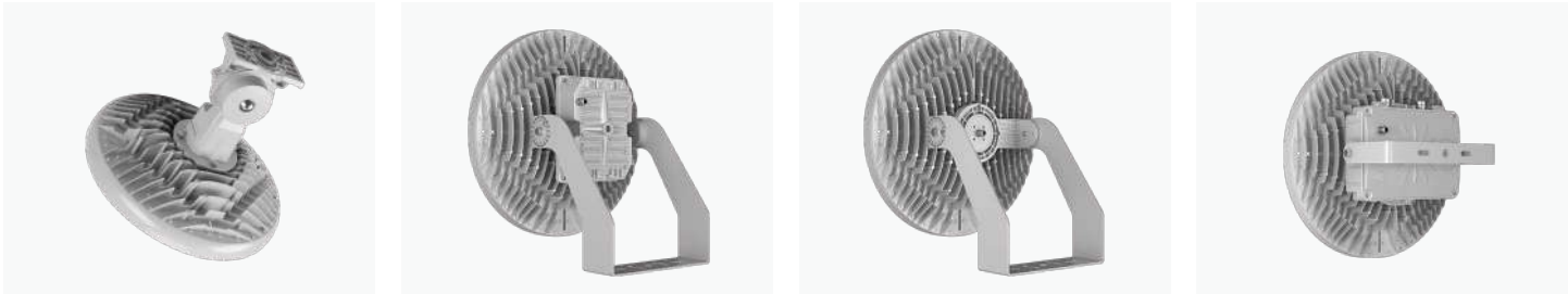
INS-A Top Fixed Installation INS-B Under Mount Yoke (with driver box) INS-C Under Mount Yoke (split mode) INS-D Yoke Mount
