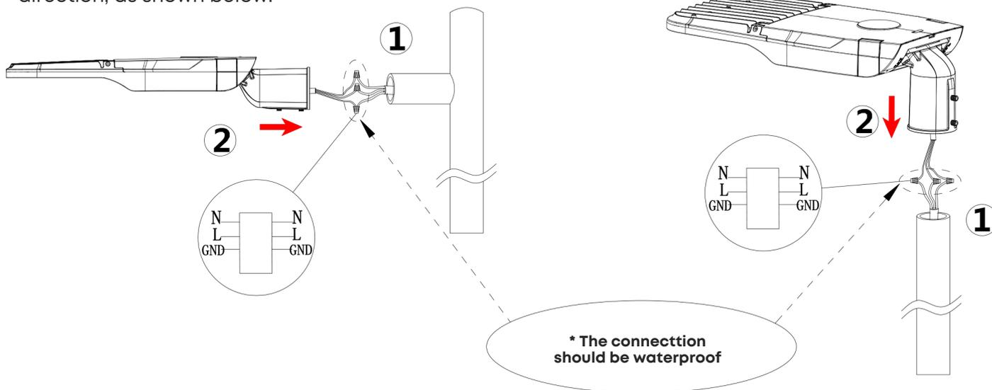
Diagram of correct and incorrect fixation of lamp pole and bracket.
