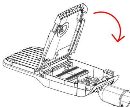
3. Place the latch correctly in the groove on the rear cover.
