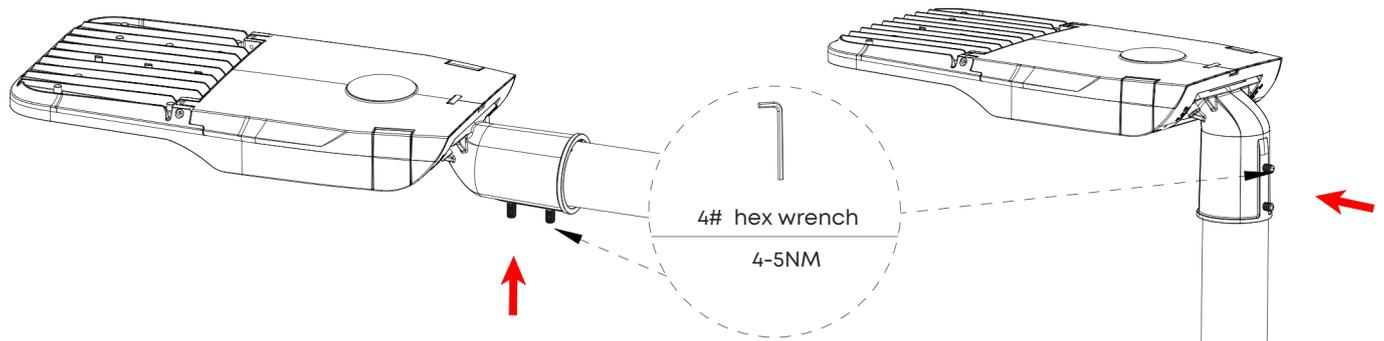
4. If angle adjustment is required, loosen the two screws by 2-3 turns, ensuring they are not completely removed. Proceed to align the component before retightening.
