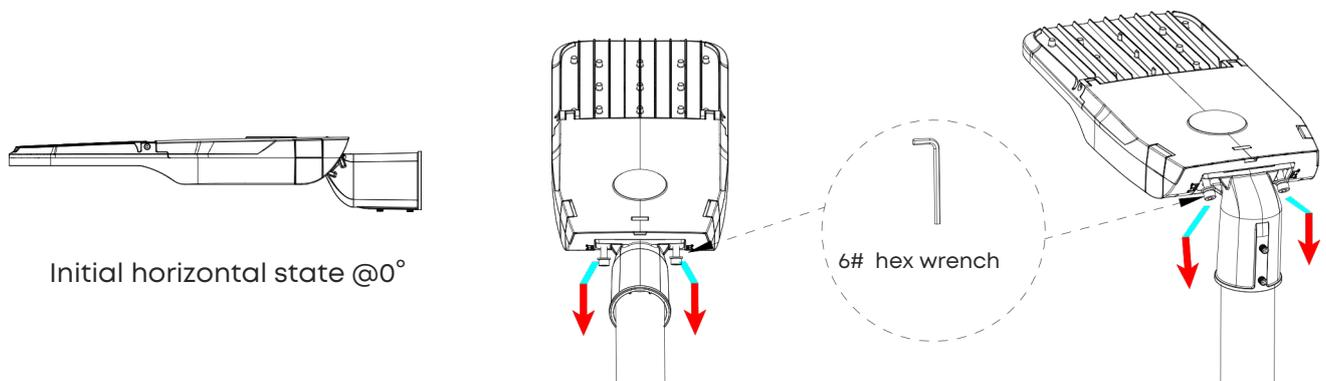
5. Rotate the fixture to the proper angle based on the actual requirement, then tighten two screws behind the fixture on the bracket.
