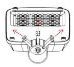
2. Connect the lamp with wire from pole (correspond L, N, GND lines), then according to the arrow direction of the lamp bracket inserted into the lamp pole (can be used on 40-63mm light poles), as shown below.
