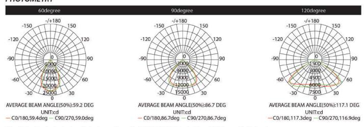
All published Luminaire photometric testing performed to IESNA LM-79-08 standards by a NVLAP accredited Laboratory.
