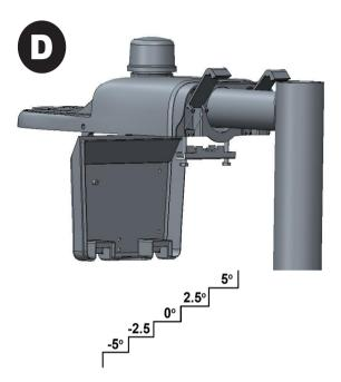
Step4-Insert the pole and adjust the angle as needed. (Figure D)
